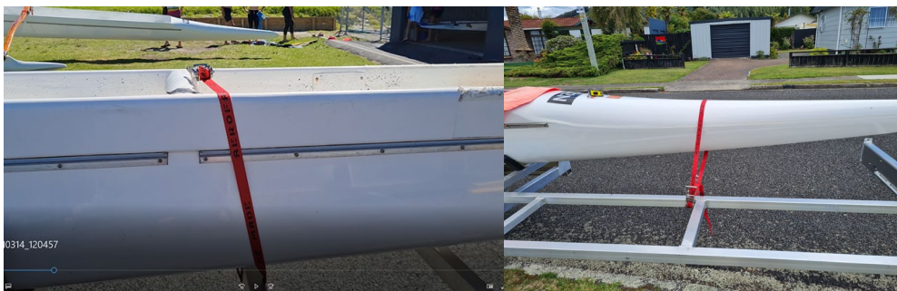
Figure 1 - Ratchet position at Taumanu - Ratchet over top of hull opening, avoid ratchet against hull surface.
